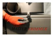
3. Attach the main container on the top of the grid and pin up with the provided screws.
