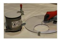
1. With the provided allen wrench remove the screws
