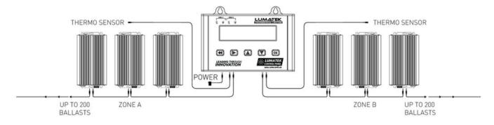
Each Zone must utilise the same fixtures in-line; e.g. Zone 'A' must be all 600w, and Zone 'B' all 630w fixtures.
