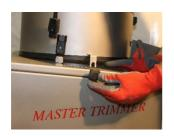
1. Attach the main cointener on the top of the grid with the screws.
