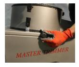
2. Screw the screws to pin up the main cointaner and connect the engine on the top to the electrical circuit.
