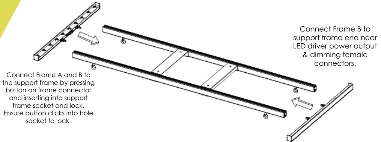
**Note the direction when installing; the LED driver mounting bracket is on top when the fixture is hung.**
