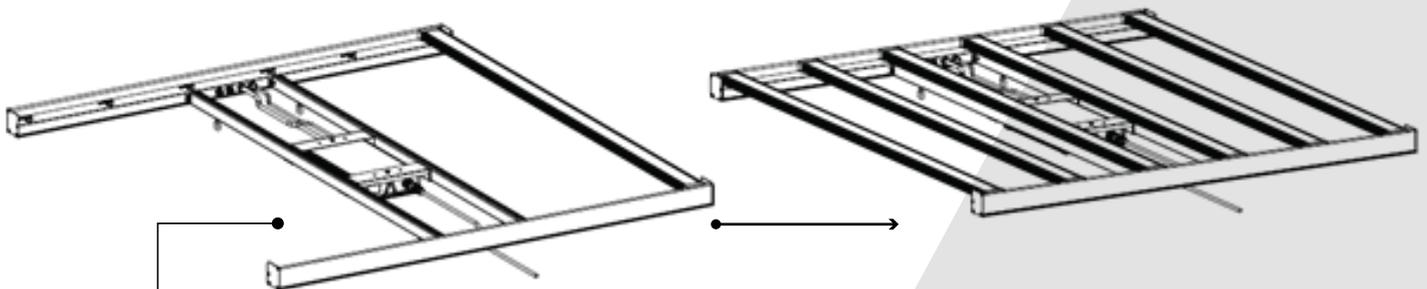
Assemble the rest of the light bars into the fixture frame as shown in the figure above.
