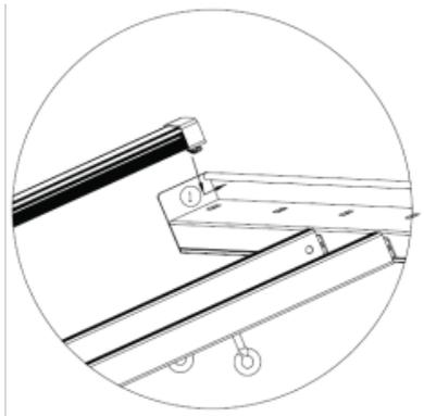
Ensure the driver is secured and flip the fixture over so the driver is now underneath. Insert the end of the light bar with the hook into the square hole in Frame A
