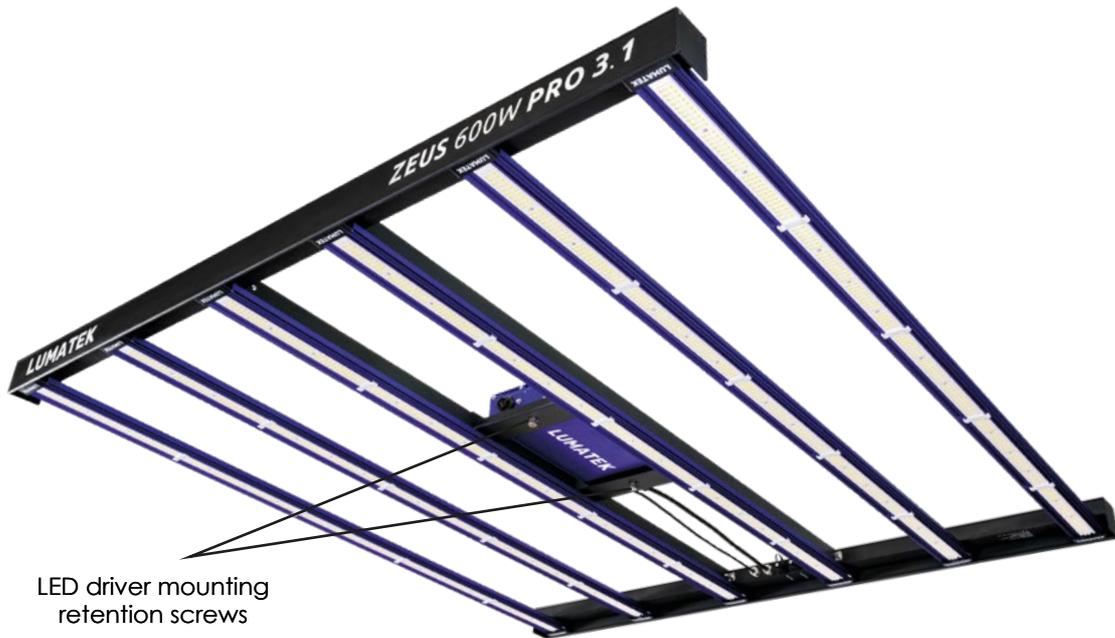
The LED driver is fixed to the mounting bracket with two retention screws through bracket into driver base plate. For greater flexibility the driver can be disconnected from the fixture and used remotely using Lumatek 5m LED driver extension cables (sold separately).
