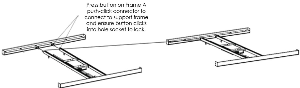
**Note the direction when installing; the driver tray is on top when the fixture is hung.**
