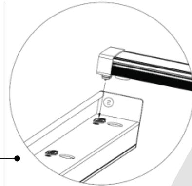
Then insert the other end; align the round hole on Frame B with the light bar's magnetic end and insert male pin into female socket. Ensure magnetic connection is secure.
