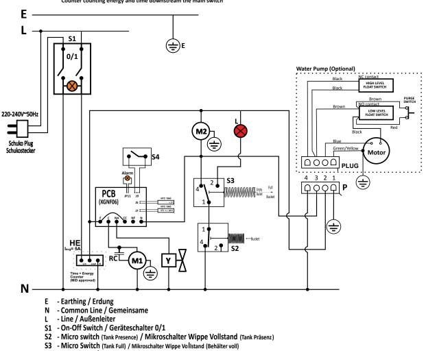
Wiring diagram with tank present & full tank & condensates pump reseting the PCB Counter counting energy and time downstream the main switch
