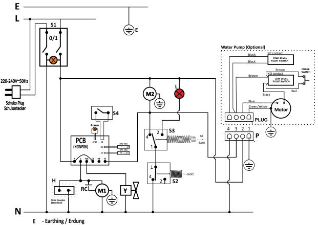
Wiring diagram with tank present & full tank & condensates pump reseting the PCB Hour counter just counting the compressor operation time
